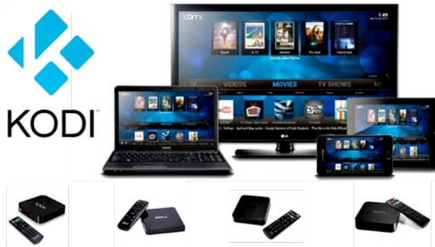
Fig. Small players, nowadays already with multi-core processors and with implemented KODI player may be connected to both LAN network or through WiFi. You may use them to build an interesting multiroom assemblies controlled directly by Foxtrot.
