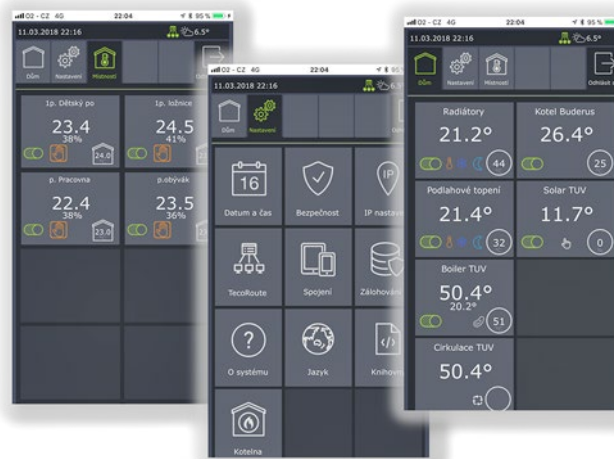
Fig. An application in a mobile telephone allows clear and detailed display and control of each room. It may also be used to configure other service and user settings. It also works as a multi-WiFi thermostat accessible through the Internet.
