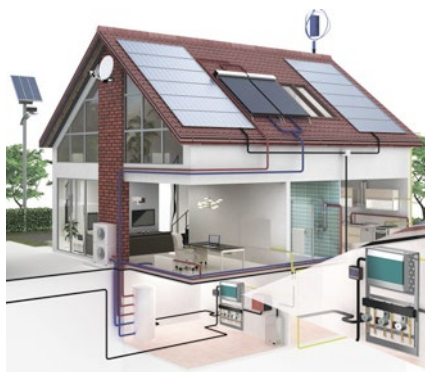
Fig. A typical heat distribution system – the installation of circulating pumps and control valves for multi-circuit heating system is reduced thanks to RITbox, which only requires the technician to connect pipes to a compact unit mounted on the wall.
