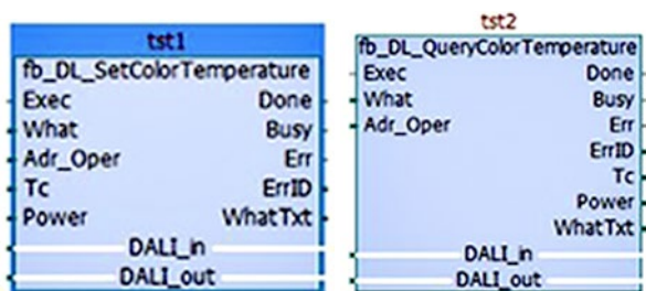
Fig. Picture for programmers – functional blocks from the DALILibPlus library used for light chromaticity temperature control.
