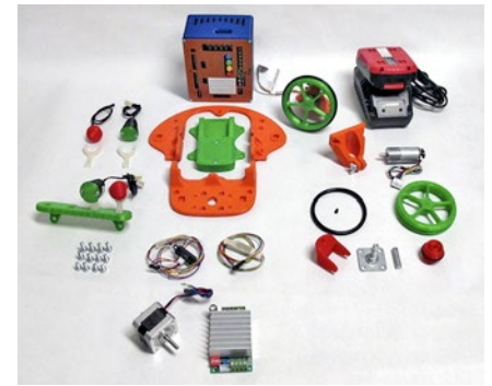
Fig. Foxee robot kit with 3-D printed parts
