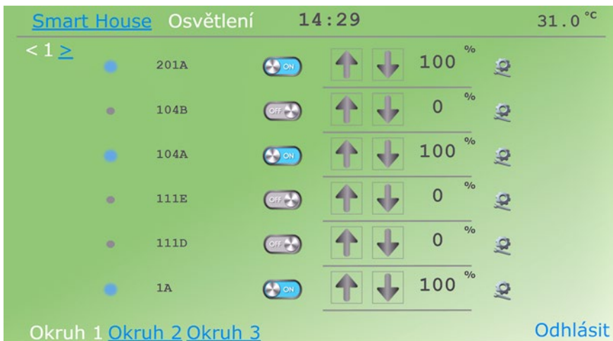
Fig. Home screen of the Smart Control system allows you to control all technologies installed in the house, monitor their status and take manual actions based on your own decision but also to configure logic, quantitative and time requirements for fully automated behavior of the entire house.
