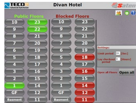
Fig. Control windows/pages of the elevator access system in Divan hotel. These were created in Mosaic environment and run directly on the Foxtrot hardware.
