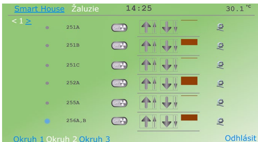
Fig. The picture shows the position of each blinds in relation to the window. Functional conditions for each blind may be set individually.
