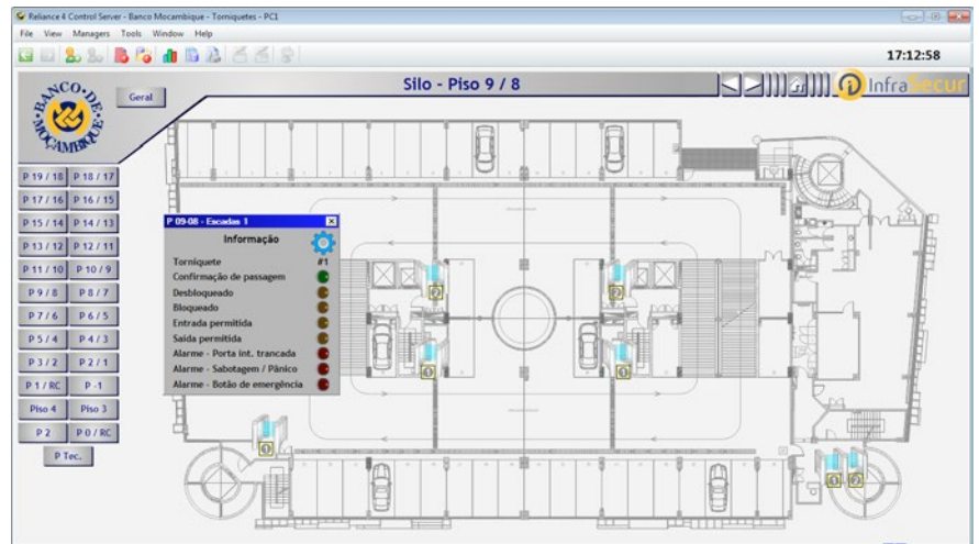
Fig. The control and overview diagram of the bank access system was created by InfraSecur in SCADA Reliance.
