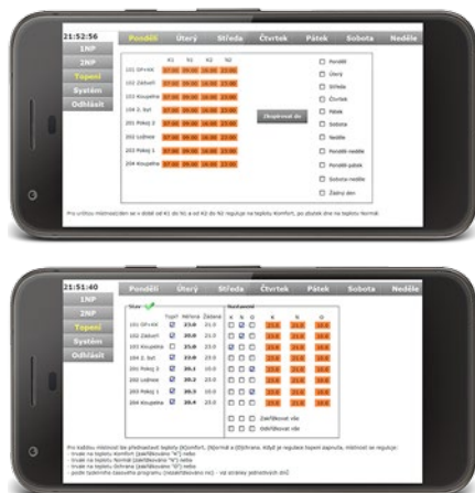
Fig. To correctly configure multiple weekly schedules for several rooms including different temperature requirements you need to use more complex multi-table input screens.
