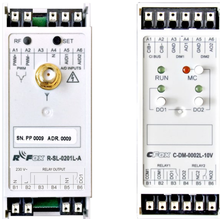
Fig. Modules used for dimming one to two ballasts used in public lighting system. C-DM-0002L-10V is a two-channel unit on CIB bus (for 2 ballasts), and the R-SL-0201L-A is a single channel unit connected to the Foxtrot CPU wirelessly using frequency of 868mHz. It has two inputs for external sensor and an internal detector which detects the primary current necessary for diagnosing the LED chip function on the secondary side.
