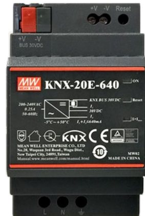
Fig. The KNX-20E-640 power supply module is able to supply the KNX network with up to 640mA. Therefore, a full-featured extension of the Foxtrot basic module with the KNX network will occupy a total width of 4 modules in the cabinet.
