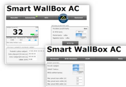
Fig. 4 Parameters of each individual wall box in the interconnected arrangement are configured separately through online application.
