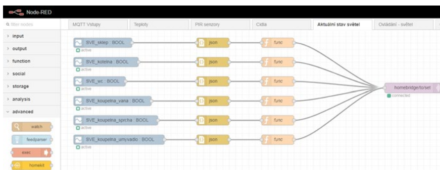
Fig. A sample showing how to use Node RED functional blocks to connect lamps controlled by Foxtrot into HomeKit platform made by Apple.
