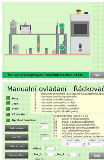
Fig. Interactive control screens of the touch panel clearly depicting the actual machine. Parameters are entered in the tables, which also offer text-based assistance.
