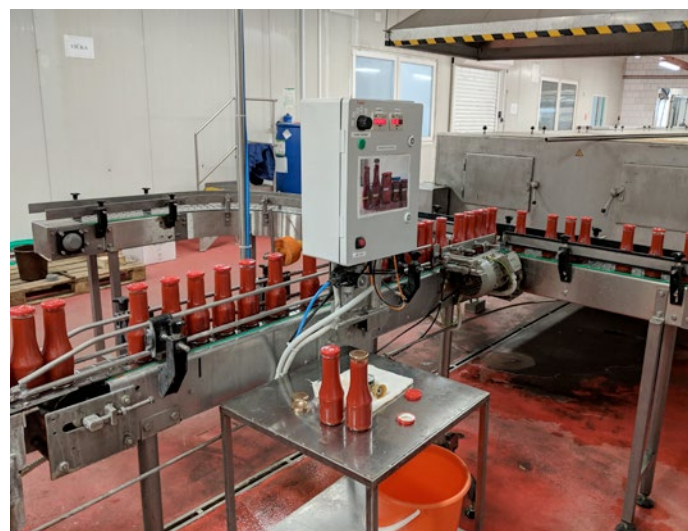
Fig. Another implementation of an inspection station which is used to check the hermetic seal by utilizing Tecomat Foxtrot system. This time the check station is installed on a line that is used to produce ketchup bottles.
