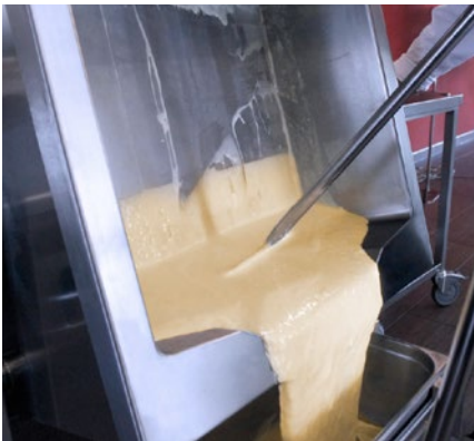
Fig. 2 the multifunctional equipment is also supplied with a function able to accomodate a pressurized system. Just connect it to the electric power and to water and waste pipes. the cook only introduces the ingredients and then takes out the finished meal; other routine activities such as the control of temperatures and energies is handled by Tecomat Foxtrot
