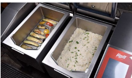
Fig. 2 the multifunctional equipment is also supplied with a function able to accomodate a pressurized system. Just connect it to the electric power and to water and waste pipes. the cook only introduces the ingredients and then takes out the finished meal; other routine activities such as the control of temperatures and energies is handled by Tecomat Foxtrot
