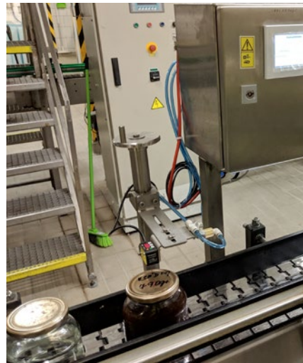
Figure. Laser detection unit monitors the quality of the seal on the final glass containers. the detection unit is installed near the conveyor belt. the evaluation is done by Tecomat enclosed in a small distribution box equipped with a touchscreen just above the conveyor belt.
