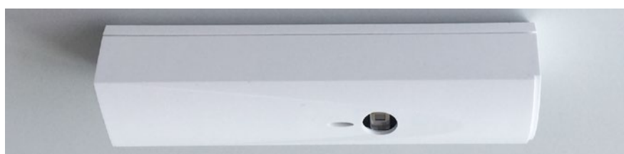
Fig. C-IF-6400R module is supplied in a plastic casing allowing installation onto the ceiling for example. It monitors the presence of persons below the sensor. It uses the application program which deals with the point metrics allowing you to deduce a lot of information. For example, the presence of the person, direction where the person came from and where the person is going, the number of persons including the direction of their arrival or exit.
