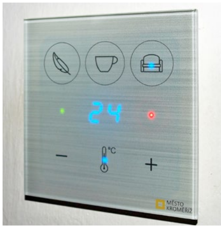
Fig. Wall-mounted touchscreen controller belonging to Touch@Glass series connected via CIB bus.
