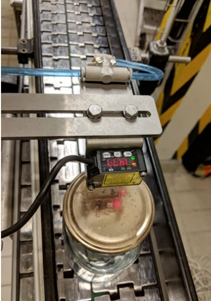
Fig. Laser unit which measures the distance or rather the deflection of the cap with the accuracy of one tenth of a millimeter, while the finished glasses pass by on the conveyor belt. the deflection of the cap is the best indicator which tells the system whether the correct seal was achieved or whether it is necessary to mark the product as defective.
